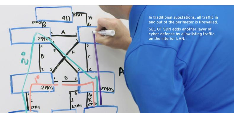
OT SDN provides strict network access control on both north-south and east-west traffic on the LAN. This provides protection against attacks which physically take place inside the firewalls and also adds protection against unauthorized traffic that slips past firewalls.
