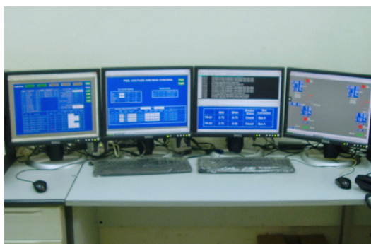
Figure 7—Remote-view stations used throughout the MOH plant allow for continuous visualization and diagnostics of the entire system.
