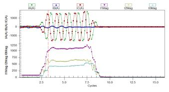
Fig. 35. Gillespie T-448 line primary relay sequence component current magnitudes
