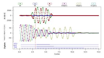
Fig. 19. Horseshoe Bay T-448 line primary relay trip output
