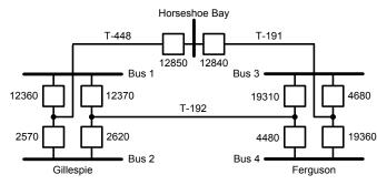
Fig. 9. System one-line diagram
