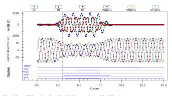
Fig. 37. Gillespie relay T-192 line replay with 87L elements
