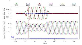
Fig. 17. Gillespie T-448 line primary relay trip output
