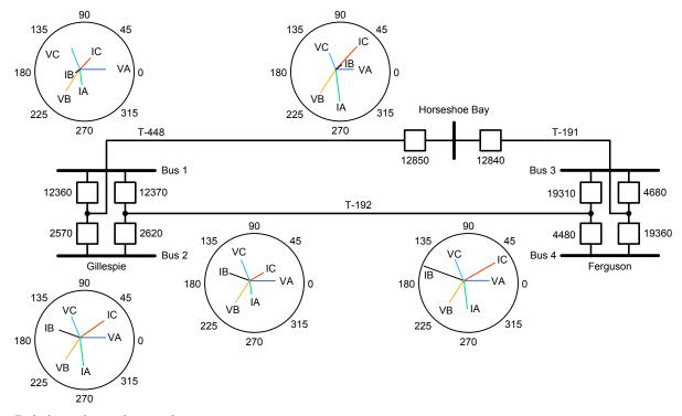
Fig. 15. Fault phase voltage and current phasors
