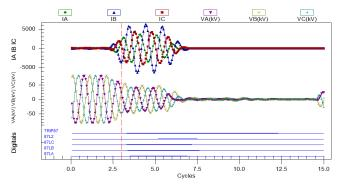
Fig. 38. Ferguson relay T-192 line replay with 87L elements
