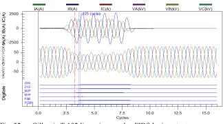
Fig. 32. Gillespie T-192 line primary relay FIDS logic output
