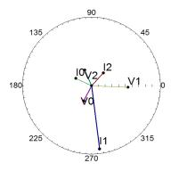
Fig. 31. Gillespie T-192 line primary relay sequence components
