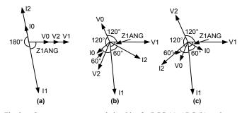
Fig. 3. Sequence component relationships for BCG (a), ABG (b), and CAG (c)  $% \left( \begin{array}{c} c \\ c \end{array} \right)$
