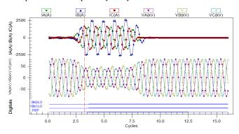
Fig. 28. Gillespie T-192 line primary relay reclose drive-to-lockout output
