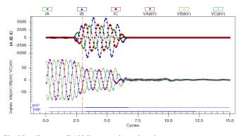
Fig. 27. Ferguson T-192 line secondary relay trip output
