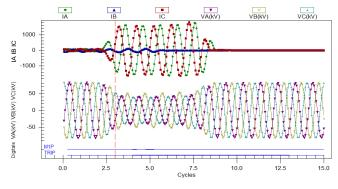
Fig. 18. Gillespie T-448 line secondary relay trip output
