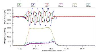
Fig. 30. Gillespie T-192 line primary relay sequence component current magnitudes
