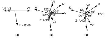
Fig. 4. Sequence component relationships for AG (a), BG (b), and CG (c)
