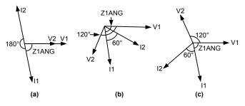
Fig. 2. Sequence component relationships for BC (a), AB (b), and CA (c)
