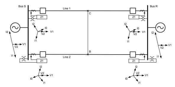
Fig. 7. BC intercircuit fault sequence voltages and current phasors
