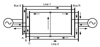
Fig. 5. BC intercircuit fault currents
