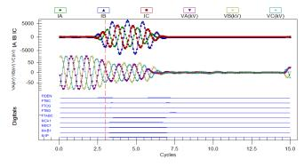
Fig. 40. Ferguson relay FIDS logic in T-192 line replay with 87L elements
