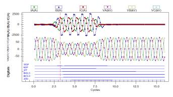
Fig. 41. Gillespie T-192 line primary relay reclose drive-to-lockout conditions
