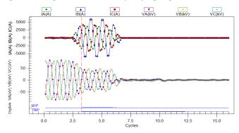
Fig. 26. Ferguson T-192 line primary relay trip output
