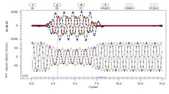
Fig. 42. Gillespie T-192 line primary relay event replay with  $a^2 = 0.4$
