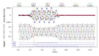
Fig. 29. Gillespie T-192 line primary relay Zone 1 distance elements
