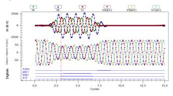
Fig. 36. Gillespie T-192 line primary relay with  $a^2 = 0.4$
