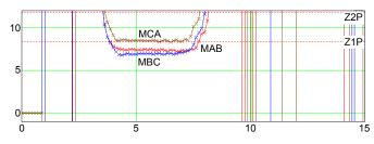
Fig. 33. Gillespie T-192 line primary relay phase distance element impedance calculations
