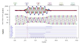
Fig. 39. Gillespie relay FIDS logic in T-192 line replay with 87L elements
