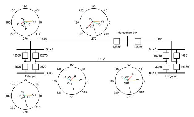
Fig. 16. Fault sequence voltage and current phasors
