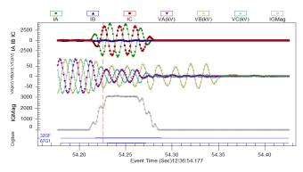
Fig. 22. Horseshoe Bay T-448 line primary relay instantaneous ground directional element
