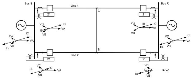
Fig. 6. BC intercircuit fault phase voltages and current phasors
