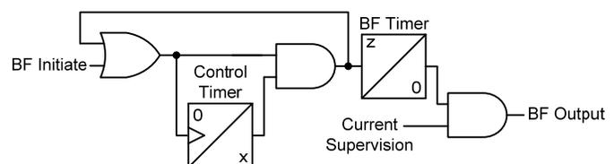
Fig. 13. Original PG&E Breaker Failure Logic
