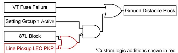
Fig. 12. Correct Single-Pole Trip for End-of-Line Switch on to Fault
