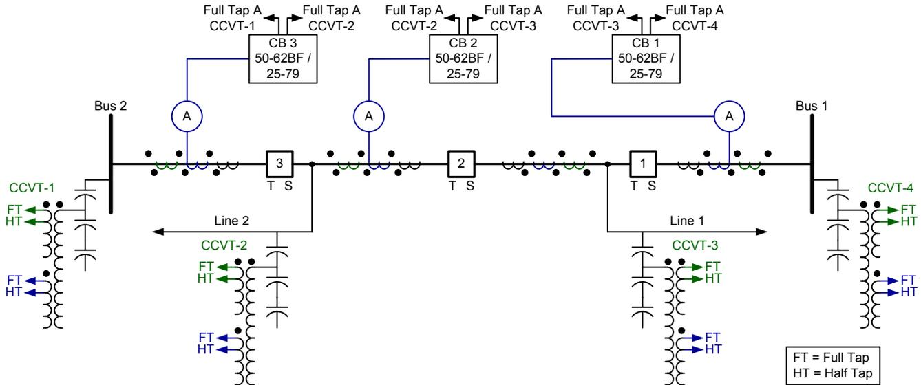
Fig. 4. Breaker-and-a-Half Breaker Relay Configuration
