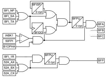
Fig. 5. Custom Breaker Failure Logic
