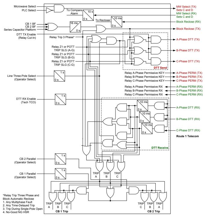
Fig. 3. DTT Integration Into Line Relays (Custom Relay Logic)
