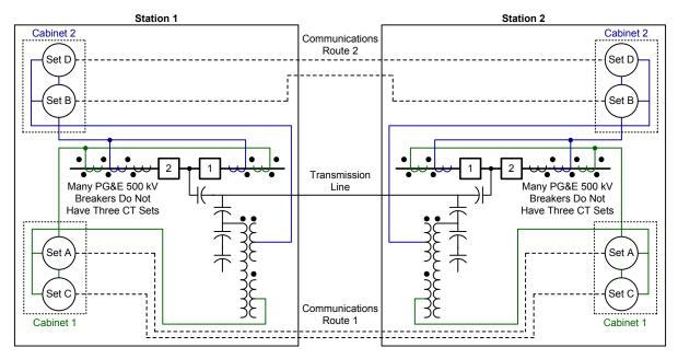
Fig. 2. Simplified Telecommunications and Relay Cabinet Design
