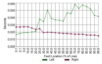
Fig. 9. Zone 2 Maximum Assertion Time for Faults Along the Line
