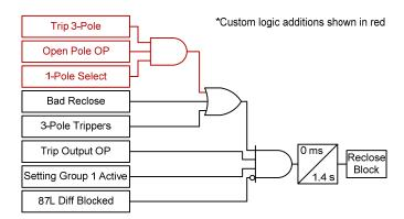
Fig. 11. Updated Custom Logic for Reclose Block for Evolving Faults
