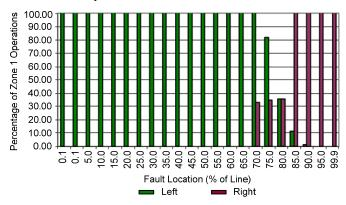
Fig. 8. Zone 1 Distance Coverage Along the Line
