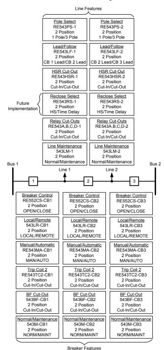
Fig. 6. Operator Interface Switches
