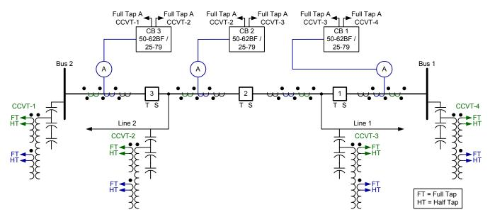
Fig. 4. Breaker-and-a-Half Breaker Relay Configuration
