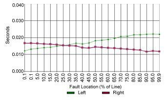
Fig. 10. Zone 2 Average Assertion Time for Faults Along the Line
