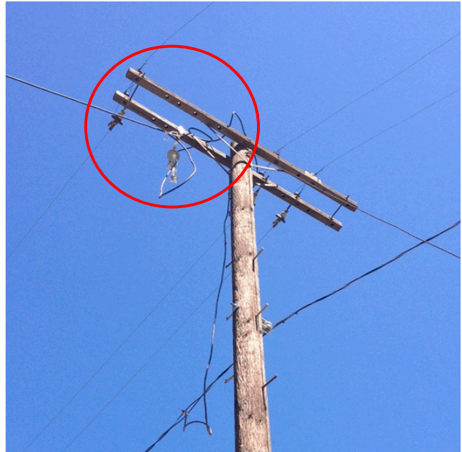
Fig. 10. A fuse link is used to create a connection between a phase on the feeder and an insulated conductor grounded at the other end. By closing the fuse link, an SLG fault is created.
