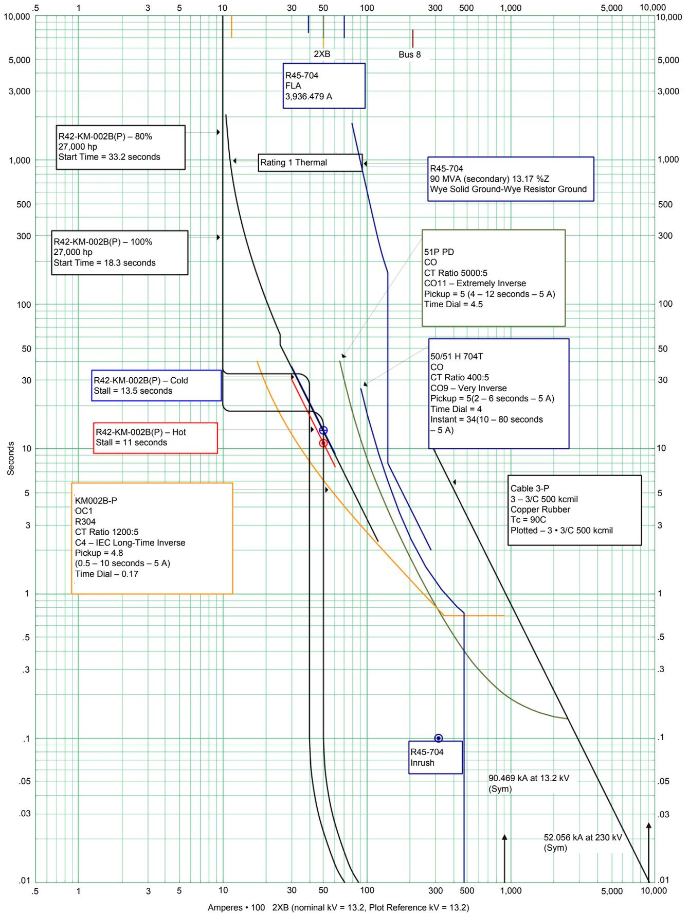
Fig. 4. 27,000 hp Synchronous Motor Curves
