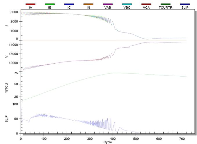
Fig. 10. 21,000 hp Motor Starting Results
