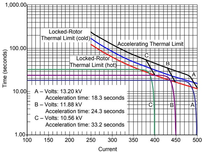
Fig. 7 Locked-Rotor Thermal Limits Versus Current
