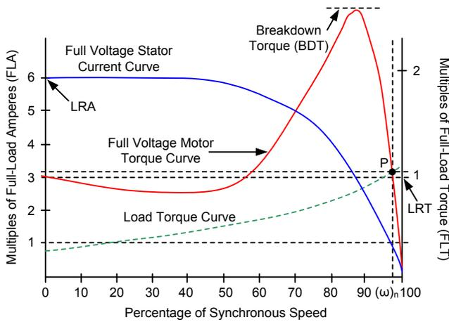
Fig. 1. Typical Motor Operating Characteristics
