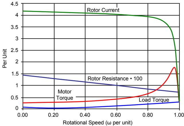
Fig. 5. Motor Starting Current and Torque
