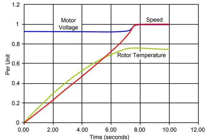
Fig. 11. 21,000 hp Motor Starting Thermal Results
