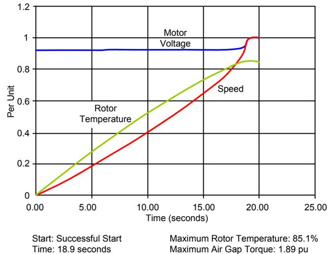
Fig. 13. 27,000 hp High-Inertia Motor Starting Example
