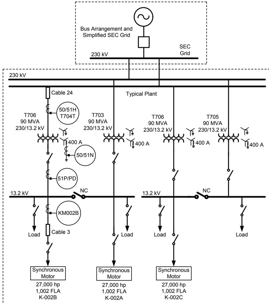
Fig. 3. System One-Line Diagram
