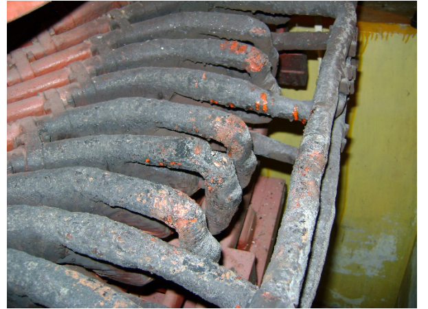
Fig. 19. Generator damage after phase-to-ground and phase-to-phase faults at different winding locations. CFE engineers in charge of fault diagnosis concluded that the fault started as a phase-to-ground fault (because of the failure pattern on the winding) and evolved to a phase-to-phase fault.
