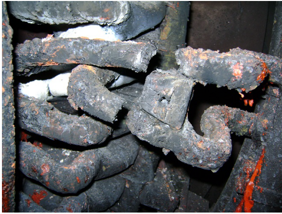
Fig. 20. Another view of the generator damage after phase-to-ground and phase-to-phase faults at different winding locations.
