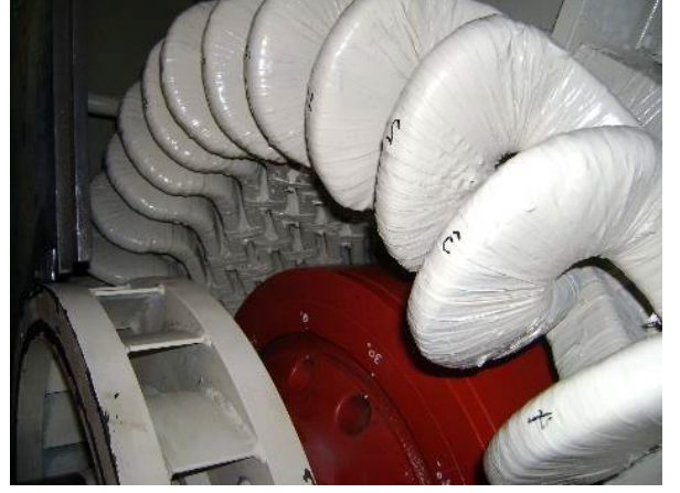
Fig. 6. A 26.6 MVA, 13.8 kV, direct air-cooled turbogenerator end.
