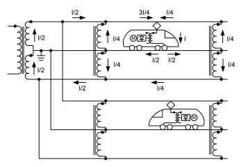
Fig. 3. 2x25 kV Railway System
