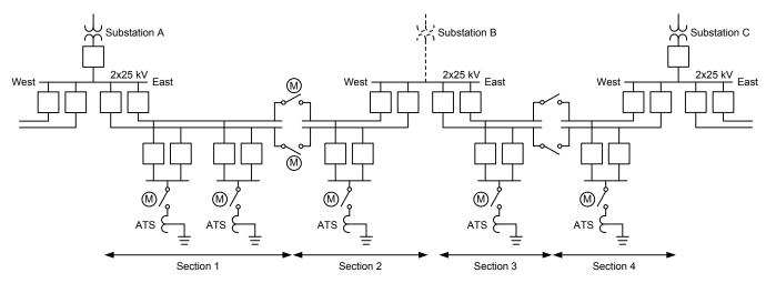
Fig. 5. 2x25 kV and Dual Rail Direction Example
