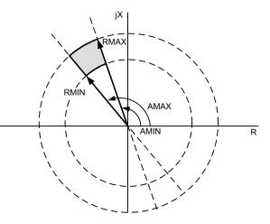
Fig. 22. Wrong Phase Coupling Impedance Area on the ZAB Plane
