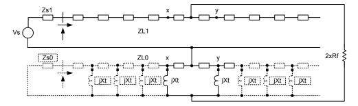
Fig. 14. Sequence Network for a Catenary-to-Ground Fault or Load Flow
