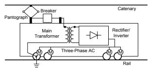
Fig. 1. The Moving Load (the Locomotive) in an Electrical Railway System
