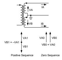
Fig. 8. Symmetrical Components in a Two-Phase System
