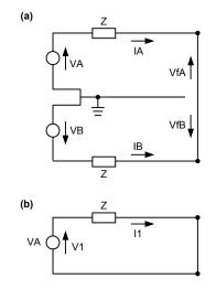
Fig. 9. Phase-to-Phase Fault (a) and Equivalent Sequence Network (b)
