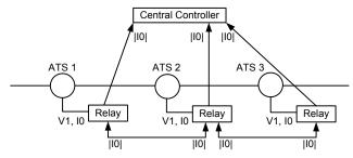
Fig. 24. Possible Architectures for |I0| Exchange for Fault Location
