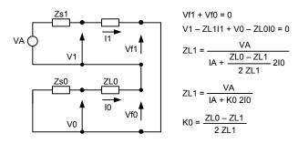
Fig. 12. Phase-to-Ground Fault Loop Impedance
