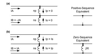
Fig. 13. Positive-Sequence (a) and Zero-Sequence (b) Autotransformer Equivalent Sequence Impedances
