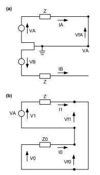
Fig. 10. Phase-to-Ground Fault (a) and Equivalent Sequence Network (b)
