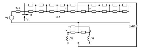
Fig. 18. Sequence Network Equivalent for a Catenary-to-Ground Fault
