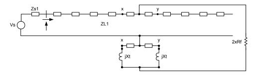
Fig. 15. Practical Sequence Network Equivalent for a Catenary-to-Ground Fault
