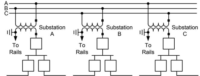
Fig. 4. Distributing Power Along the Railway Trajectory
