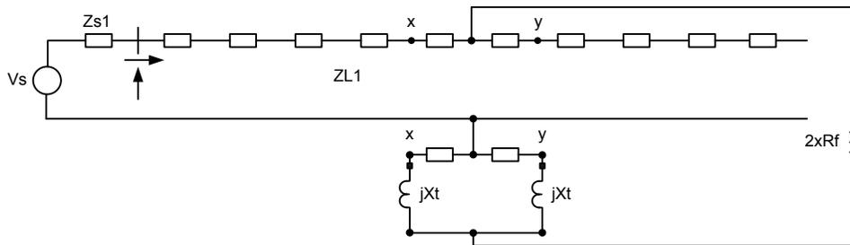
Fig. 15. Practical Sequence Network Equivalent for a Catenary-to-Ground Fault
