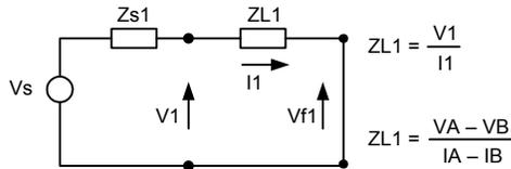
Fig. 11. Phase-to-Phase Fault Loop Impedance
