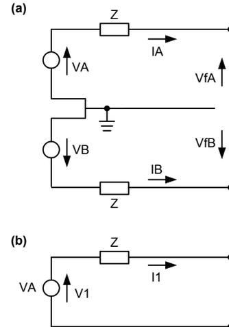
Fig. 9. Phase-to-Phase Fault (a) and Equivalent Sequence Network (b)
