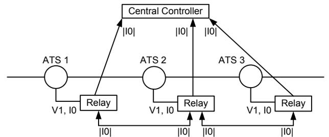
Fig. 24. Possible Architectures for  $|I_0|$  Exchange for Fault Location
