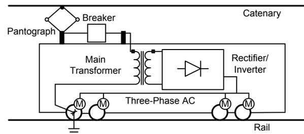
Fig. 1. The Moving Load (the Locomotive) in an Electrical Railway System
