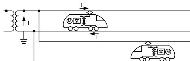
Fig. 2. 1x25 kV Railway System
