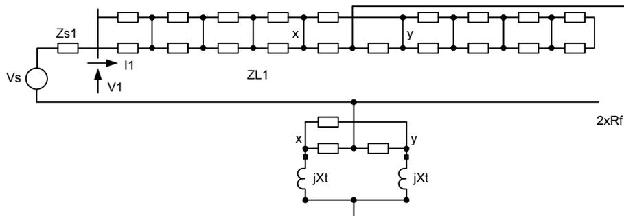
Fig. 18. Sequence Network Equivalent for a Catenary-to-Ground Fault
