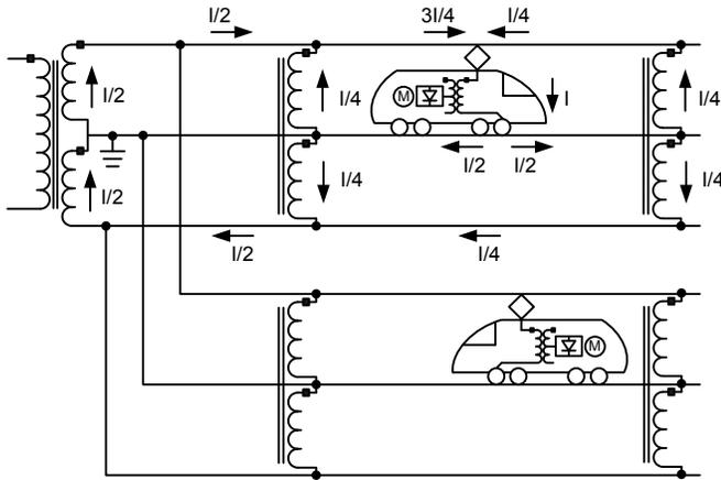
Fig. 3. 2x25 kV Railway System
