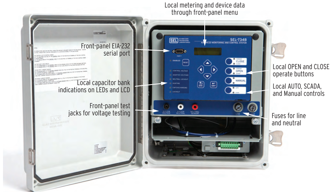
Figure 1 Compact Enclosure With Terminal Block Connector
