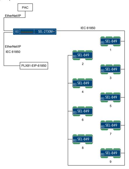
Figure 2 IEC 61850 to EtherNet/IP Network Architecture
