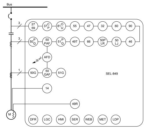
Figure 1 SEL-849 Motor Management Relay Functionality
