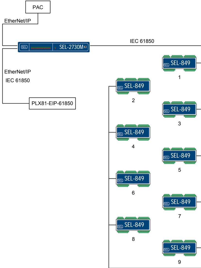
Figure 2 IEC 61850 to EtherNet/IP Network Architecture
