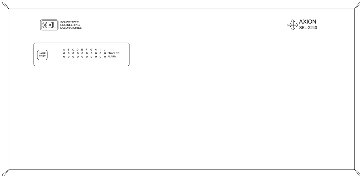
Figure 37 Figure 38 SEL-2240 10-Slot Front Panel (Panel Mount)
