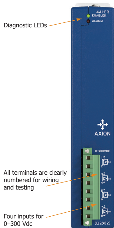
Figure 32 SEL-2245-22 Analog Input Extended Range Module Terminal-Side View
