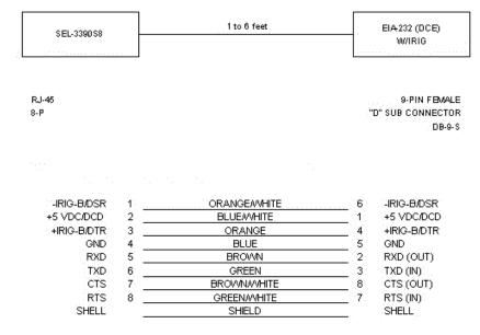
Comments: Jack Screws are attached to 9-pin female connector.
