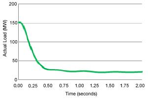
Fig. 9. Generator Runback During CGT 1 Islanding Test
