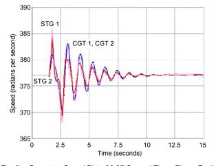
Fig. 4. Generator Speed Plot of 0.28-Second Three-Phase Fault
