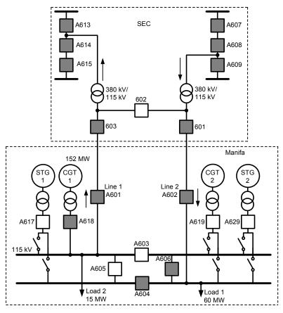
Fig. 13. System Configuration Before Remote-End Trip
