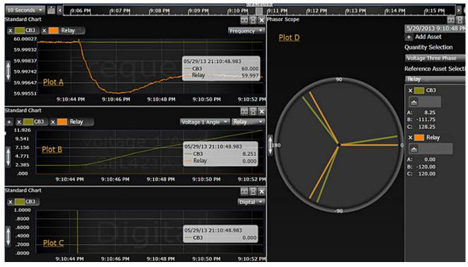
Fig. 7. Synchrophasor-Based Visualization (Phase Angle)
