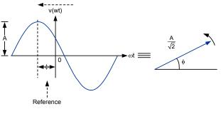
Fig. 2. Sinusoidal Voltage Time Waveform and Phasor Presentation
