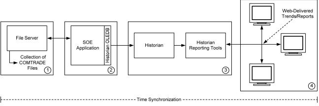
Figure 12. Oscillographic file consumption
