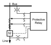
Figure 1. Protection one-line diagram for a feeder relay
