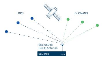
Satellite signal verification—the SEL-2488 and SEL-9524B GPS/GLONASS GNSS Antenna receive signals from two satellite constellations to validate GPS time signals, providing a layer of protection from GPS spoofing attacks.
