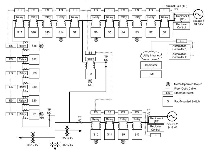
Fig. 1. The UDAS Architecture
