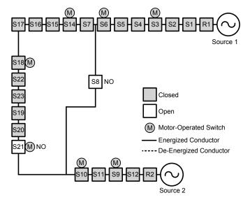
Fig. 5. Example Idle Step
