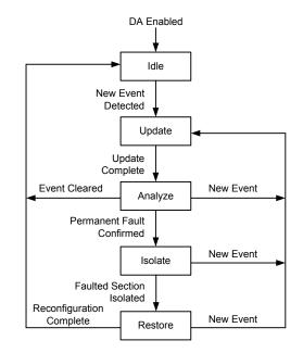
Fig. 4. Automatic Reconfiguration Sequence
