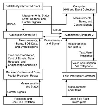
Fig. 2. System Information Flow Diagram
