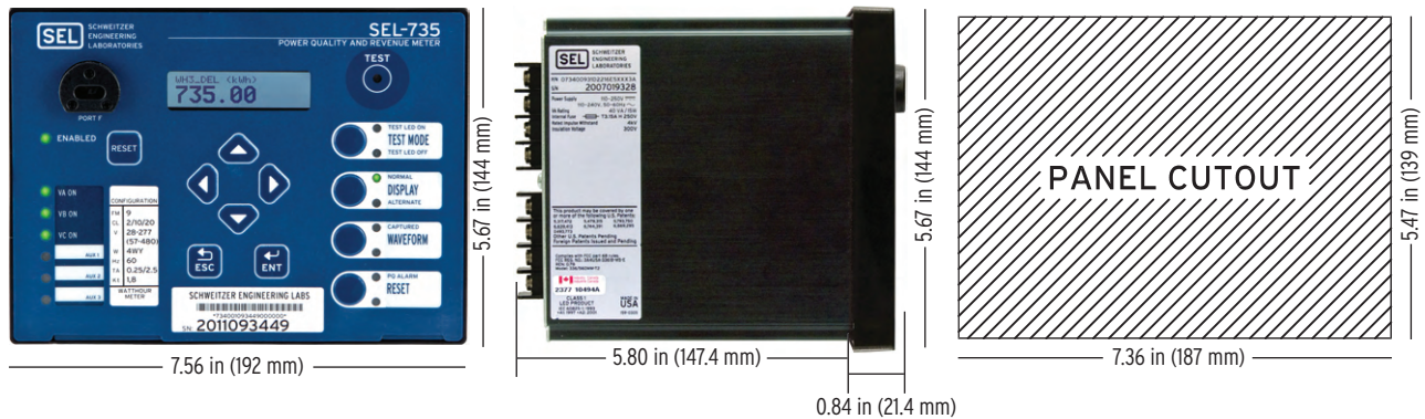
Figure 24 SEL-735 Horizontal Dimensions
