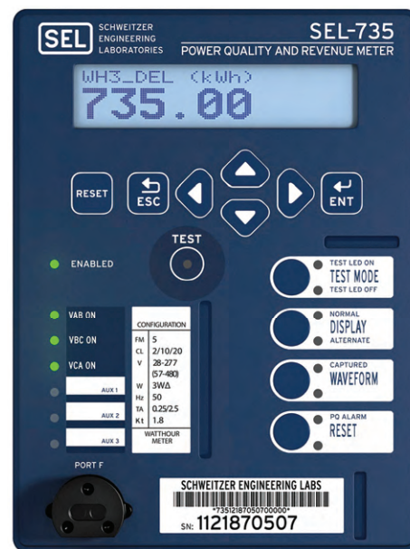
Formattable 1- and 3-line monochromatic LCD display model
