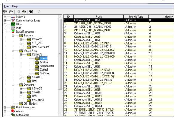
Figure 2 Data Exchange Virtual Remote Terminal Unit (RTU) Data Set With Points to Serve to SCADA Center
