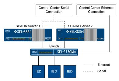
Figure 1 SCADA Server Based on SEL-3354 and Survalent SmartGateway Software
