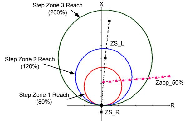
Fig. 10. Mho ground distance elements at Bus R.
