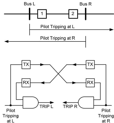
Fig. 4. Permissive overreaching transfer trip logic.
