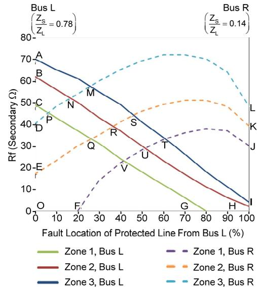
Fig. 11. Fault resistance coverage with remote end closed.
