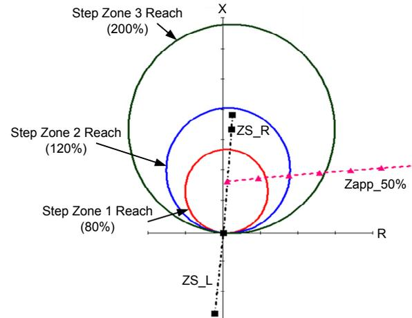
Fig. 9. Mho ground distance elements at Bus L.
