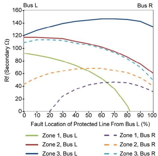
Fig. 12. Fault resistance coverage with remote end open.
