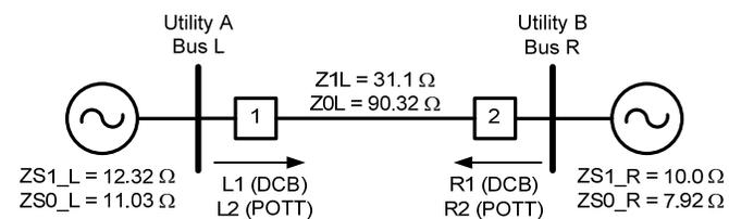
Fig. 15. Protected transmission line for Case 2 (all values are in primary ohms).
