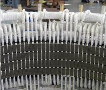
Fig. 8. An illustration of how the stator coils are braced and wedged in a large synchronous machine.
