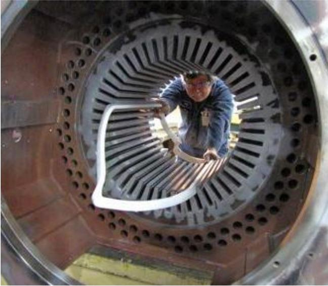
Fig. 5. Insertion of a form-wound coil winding into a small synchronous motor.
