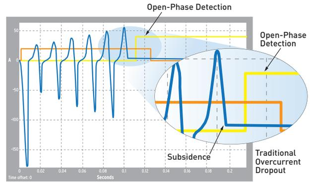
High-speed, open-pole detection logic detects open-pole conditions in less than 1 cycle to reduce breaker failure coordination times.
