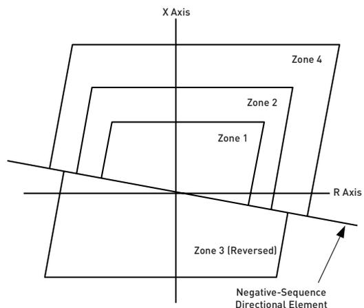
Quadrilateral Ground-Distance Characteristics
