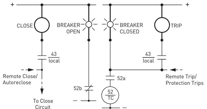
Optional trip/close pushbuttons operate independently from the relay function.
