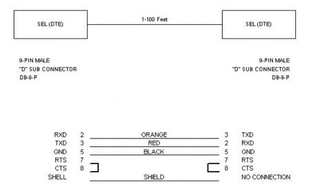
Comments: C272R cable uses metal connector shells for improved shielding.
