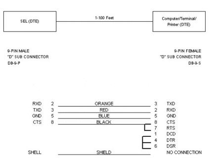
Comments: C234R cable uses metal connector shells for improved shielding.
