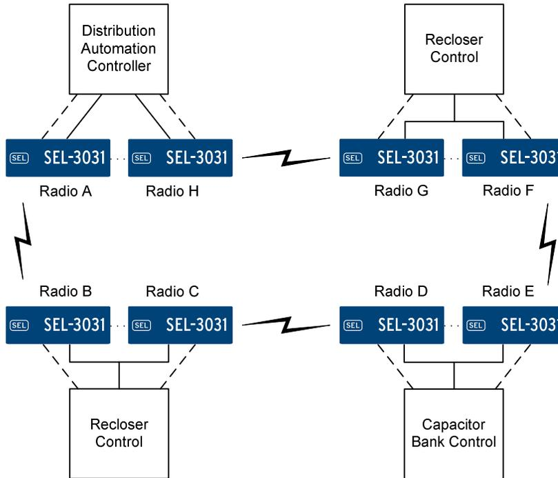
Figure 3 Distribution Automation Solution
