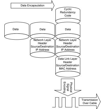
Fig. 3 Simplified Data Encapsulation and Transmission
