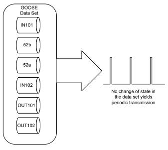
Fig. 6 GOOSE Message With Periodic Transmission
