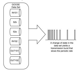
Fig. 7 GOOSE Message After a Change of State in the Data Set
