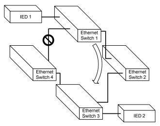
Fig. 5 Communications Path in a Simple Ring Network
