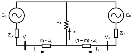
Fig. 1. Equivalent diagram of a two-terminal line with a fault at  $m$  pu from the left terminal.
