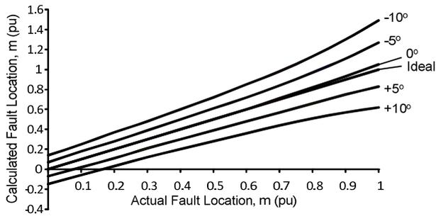
Fig. 5. Impact of phase errors in the differential signal on the accuracy of fault location using method (5) in the sample system of Fig. 3.
