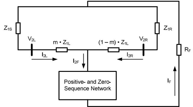
Fig. 2. Negative-sequence quantities in the sequence network for a single-line-to-ground fault.
