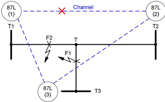
Fig. 8. Explanation of fault location reporting in master-slave configuration for three-terminal lines.
