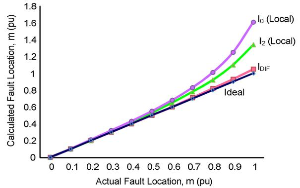
Fig. 4. Comparison of fault location results using local and differential polarizing currents.
