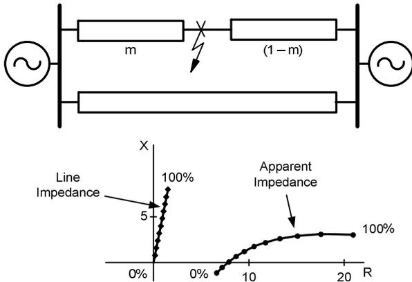
Fig. 3. Sample two-terminal system with mutually coupled parallel lines.
