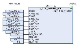
Fig. 8. CT validation function block
