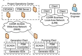
Fig. 6. PSM controller system architecture
