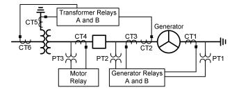
Fig. 3. Thermalito Power Plant one-line diagram
