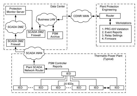
Fig. 10. System communications architecture
