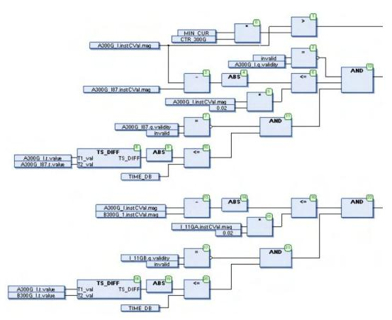
Fig. 7. CT validation function block logic
