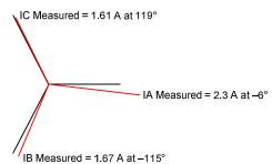
Fig. 4. In-service load readings
