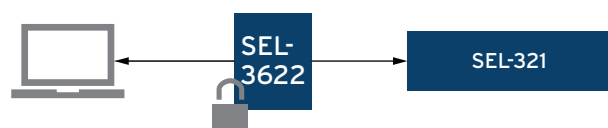
Figure 2 Protected Engineering Access
