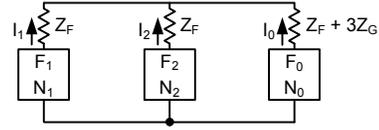
Fig. 5. Sequence network connections for a double-line-to-ground fault
