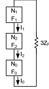
Fig. 3. Sequence network connections for a single-phase-to-ground fault
