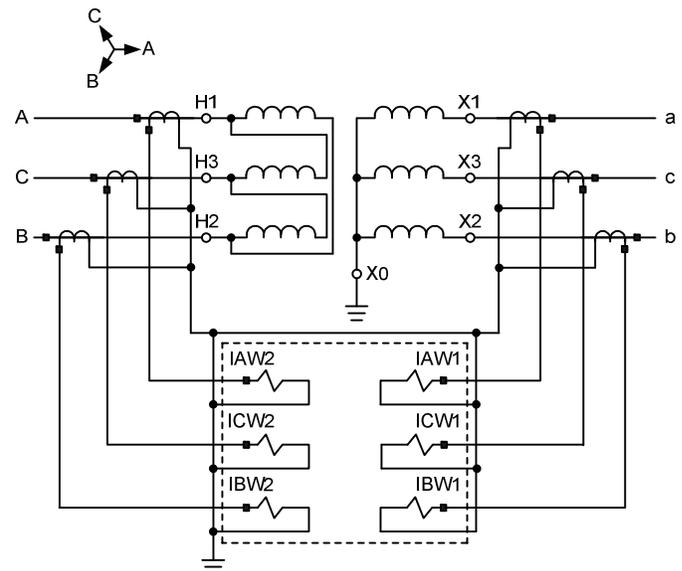
Fig. 13. Transformer phase-to-bushing connections
