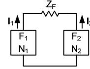
Fig. 4. Sequence network connections for a phase-to-phase fault
