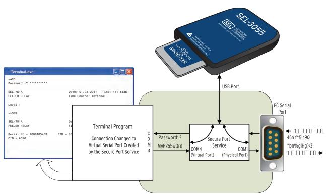
Figure 1 Serial Data Encryption Using the PC Serial Security Kit
