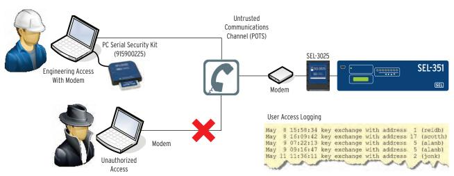
Figure 3 Secure SCADA Communications Channel
