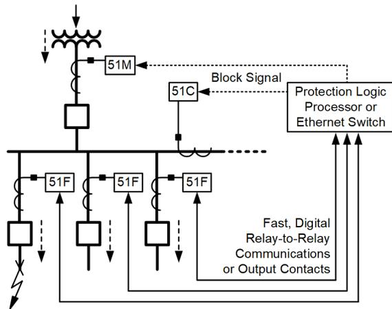
Fig. 3. Fast Bus Trip Scheme System Model With Fault on Feeder
