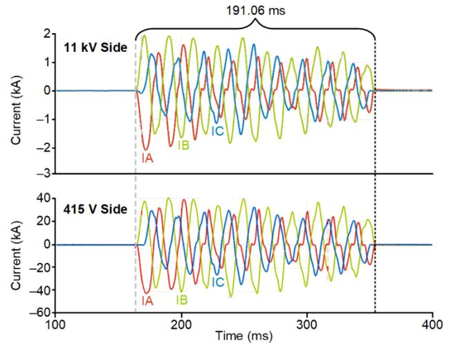
Fig. 22. Fault-Clearing Time From Event Report
