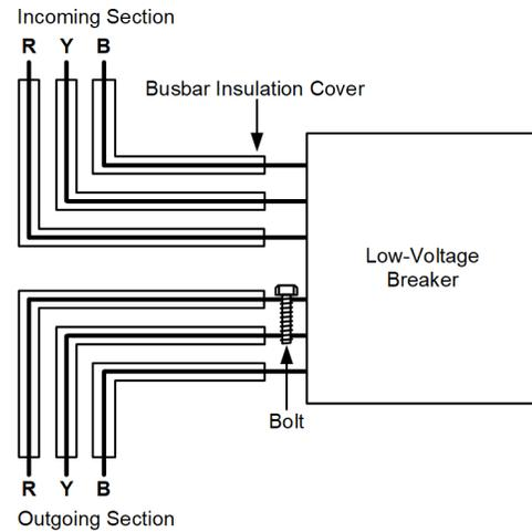
Fig. 18. Faulted Breaker Connection With Bolt on Busbar
