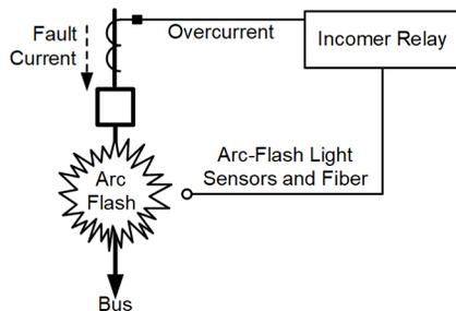
Fig. 6. Arc-Flash Detection Technology and Overcurrent Element Protection
