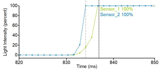
Fig. 17. Light Intensity During Arc-Flash Event
