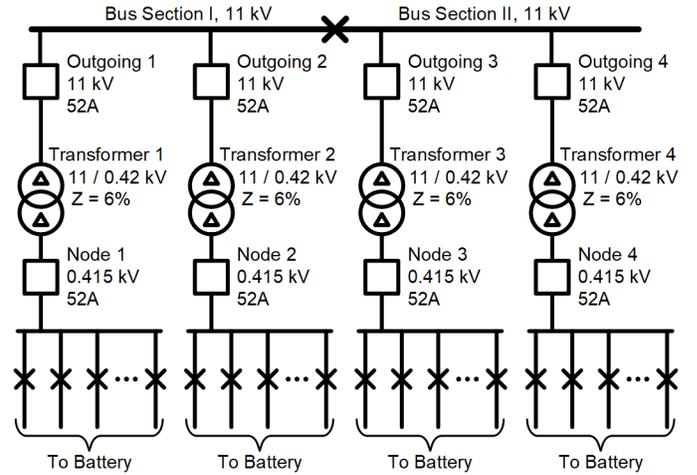
Fig. 8. One-Line Diagram of the 11/0.420 kV Switchboard
