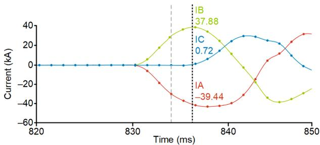
Fig. 16. Current Magnitude During Arc-Flash Event
