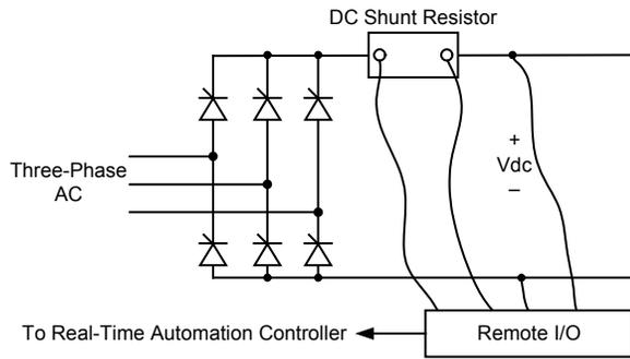
Fig. 6. Generator Field Circuit With Remote Data Acquisition
