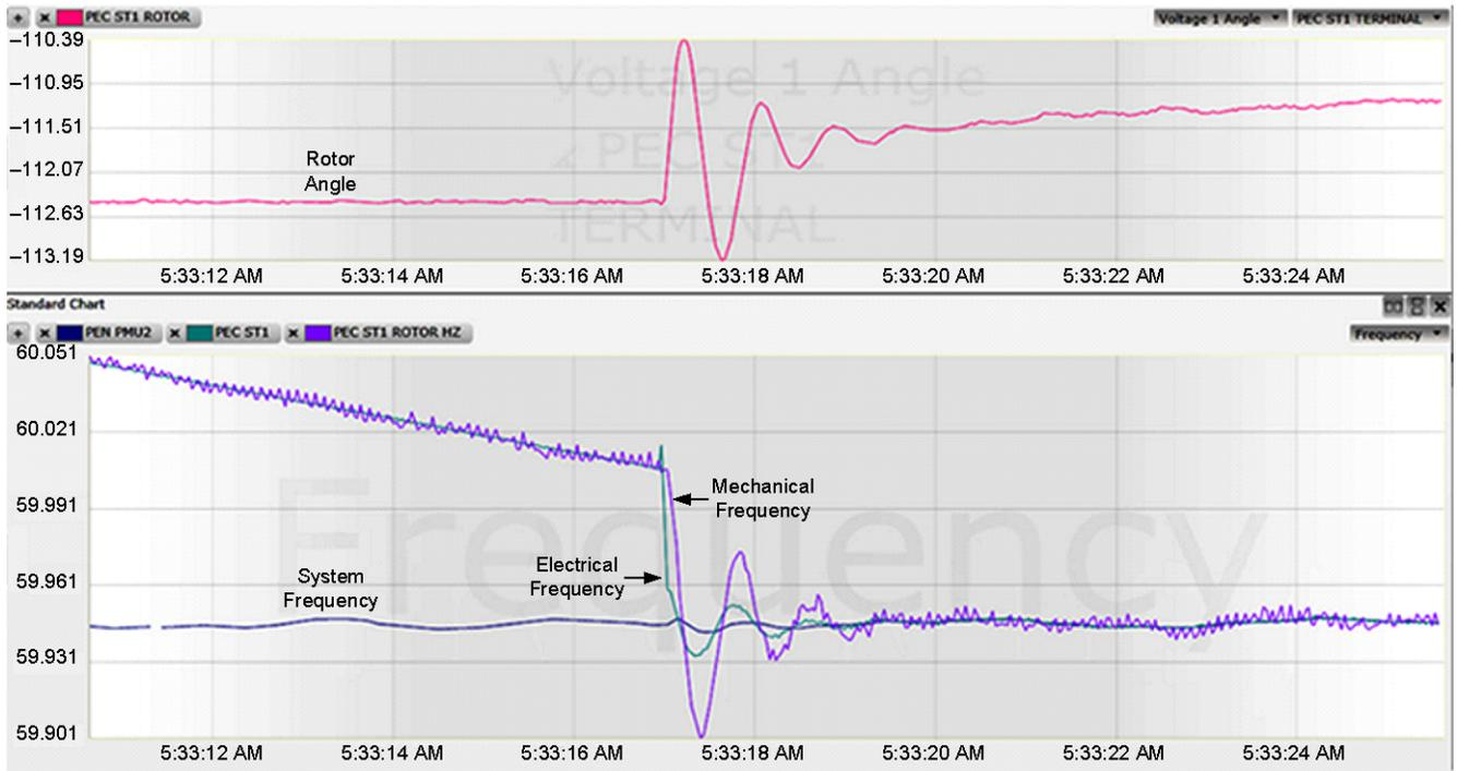
Fig. 10. Rotor Angle Capture During Synchronizing Event
