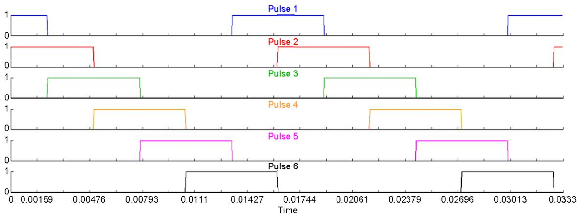
Fig. 3. SCR Gate Pulses
