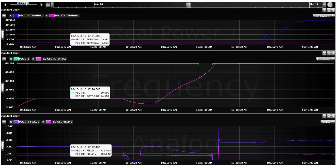
Fig. 15. Starting Curve for LCI Start
