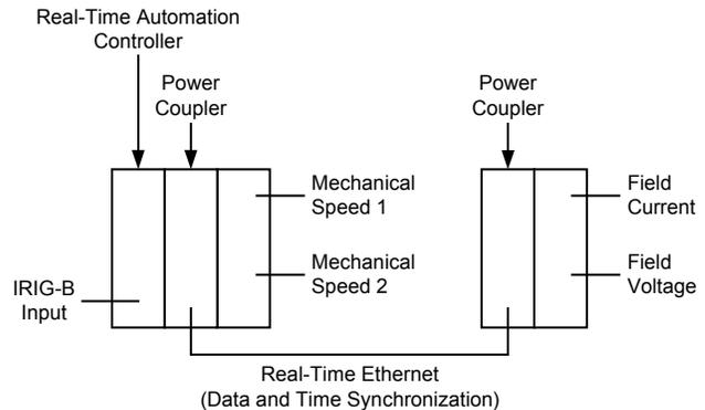
Fig. 9. Generator Monitoring System Architecture
