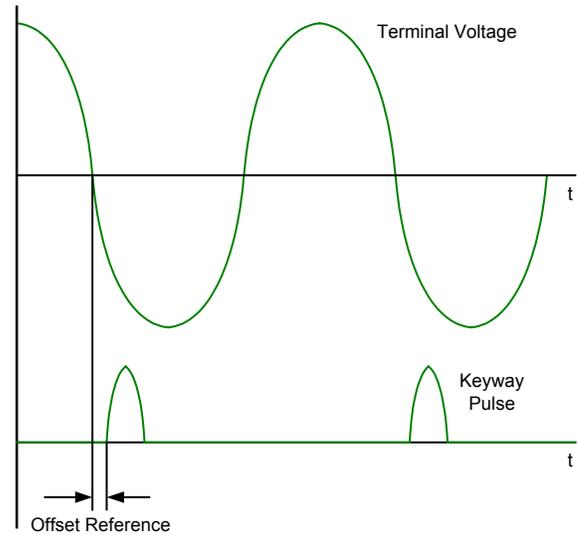
Fig. 7. Rotor and Voltage Physical Relationship
