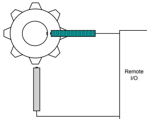
Fig. 8. Toothed Wheel Data Acquisition
