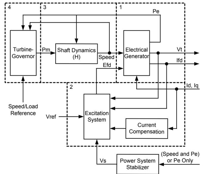
Fig. 2. Typical Generator Plant Subsystems [4]
