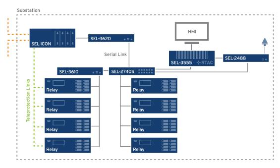
SEL communications work as a system to provide secure connectivity from the WAN to substation devices.
