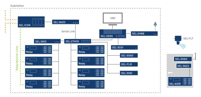
SEL wireless products extend communication to devices downline from substations, including recloser controls, voltage regulators, SEL fault and load transmitters, and more.
